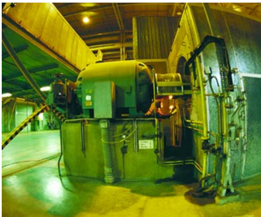
Anthony Weatherspoon checks one of the huge motors that powers the uranium enrichment process.
